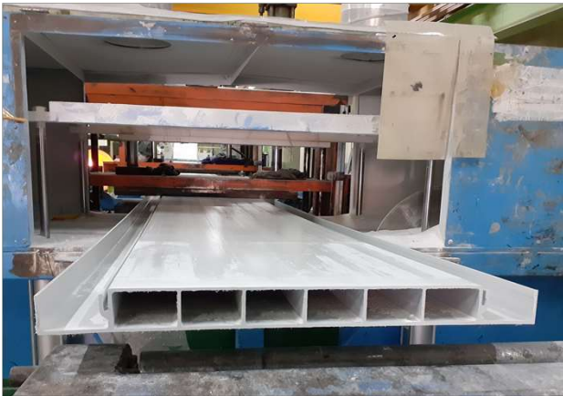
Fabrication of ISF50 Main Panel by Pultrusion
