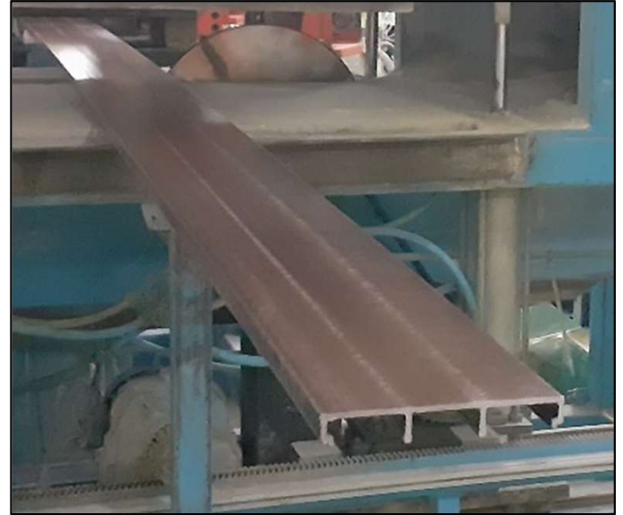
Fablication of ISF25 Lower Panel by Pultrusion
