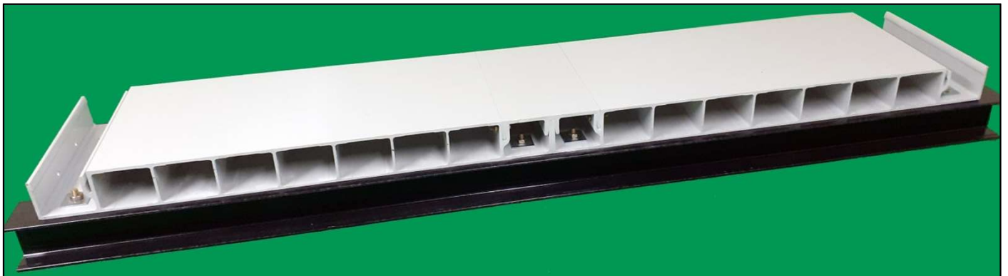
Main Panels Fixed at Girder, Bolted Each Other, Snap-Fit Interlocking with Cover Panel, Bolted at Snap-Fit, Thereby Integrally Connected in Closed-Sectional Form. Can Be Disassembled in Reverse Order
