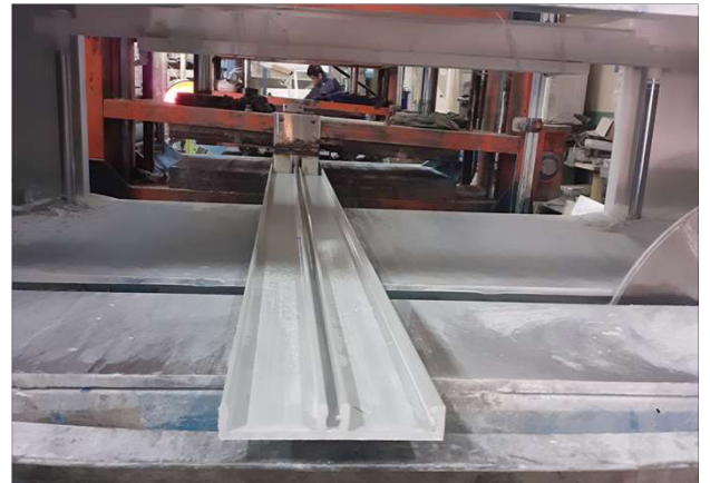
Fabrication of ISF50 Cover Panel by Pultrusion
