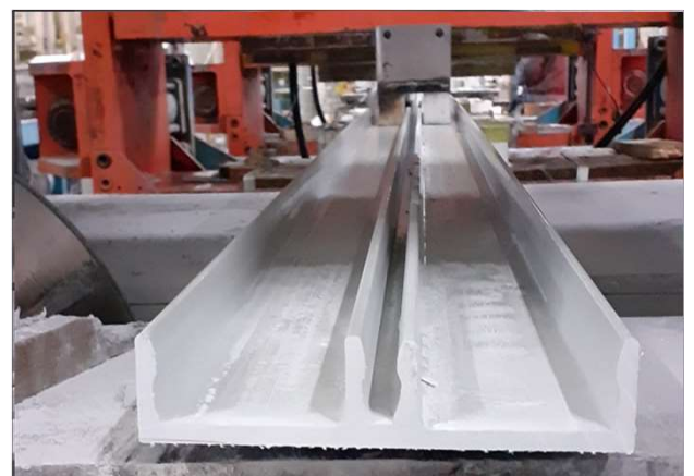
Fabrication of ISF70 Cover Panel by Pultrusion
