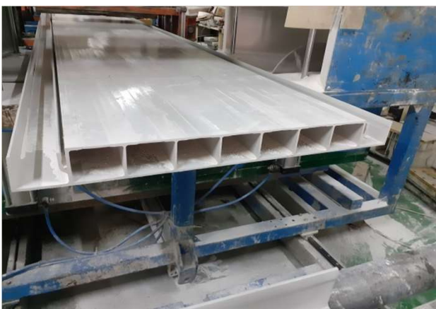
Fabrication of ISF75 Main Panel by Pultrusion
